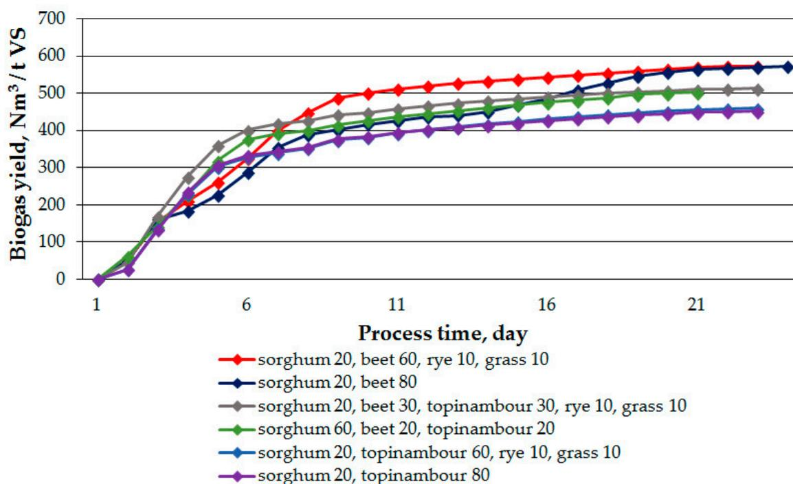
Figure 1. Biogas yield from cosubstrates on sorghum base.
