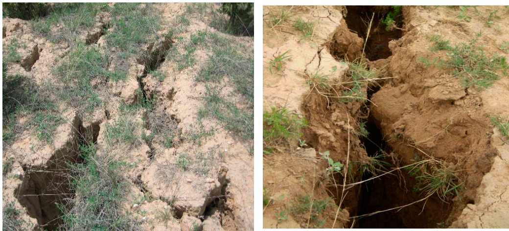
Figure 13. Surface cracks caused by goaf collapse.
