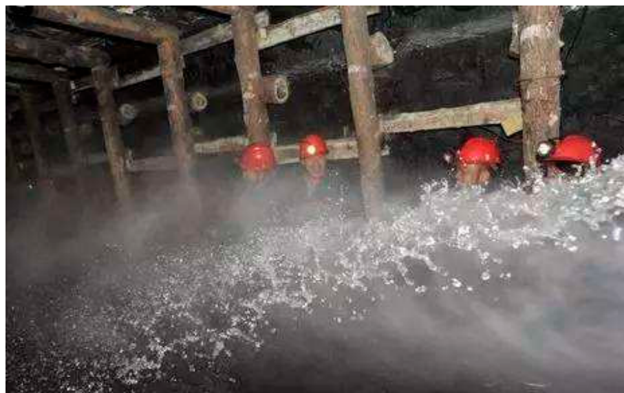
Figure 9. Water inrush accident caused by accumulated water in the goaf.
