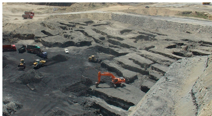
Figure 7. Recovery of the residual coal in room mining goaf by stripping.
