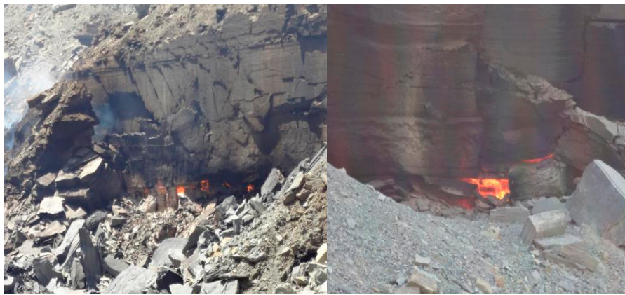
Figure 11. Spontaneous combustion of the coal seam.
