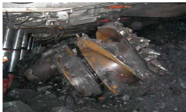
Figure 14. Rock burst of working face in the lower coal caused by stress concentration.
