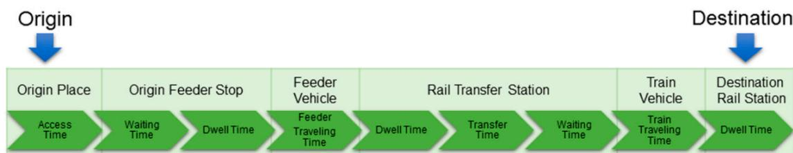
**Figure 1.** Components of travel time in both railway and feeder transit systems.
