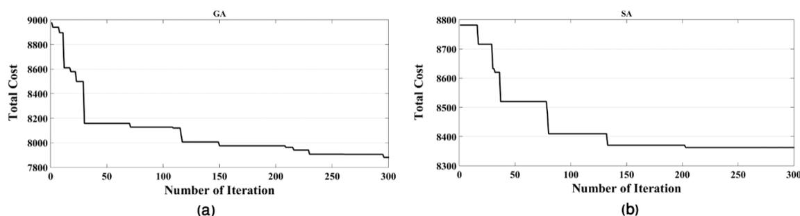
**Figure 18.** Comparison of cost history with respect to the number of iterations using: (a) Genetic Algorithm, (b) Simulated Annealing.
