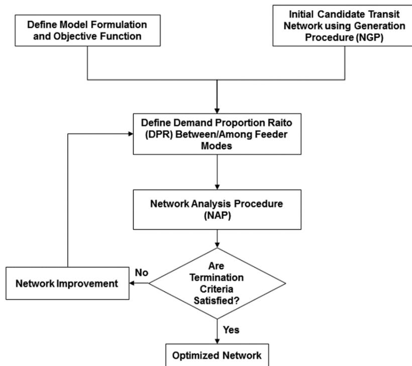
**Figure 2.** Flowchart of the solution framework for an integrated multimodal transit system.
