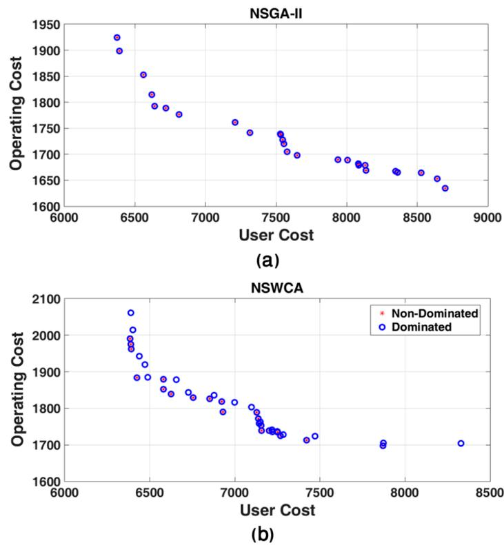
**Figure 19.** Comparison of Pareto front obtained by: (a) Non-dominated Sorting Genetic Algorithm II (NSGA-II), (b) Non-Dominated Sorting Water Cycle Algorithm (NSWCA).
