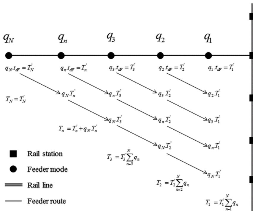
Figure 3. Condition for traveler demand in each feeder bus route linked to the railway.
