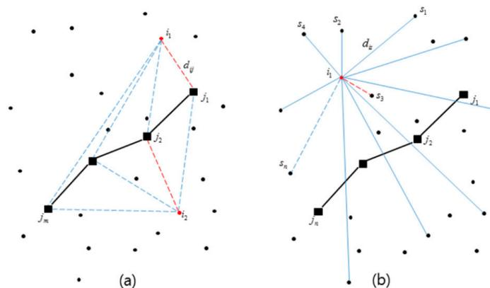
Figure 5. The initial delimiter calculation process for the: (a) station to the first bus stop; (b) bus stop to the next bus stop.
