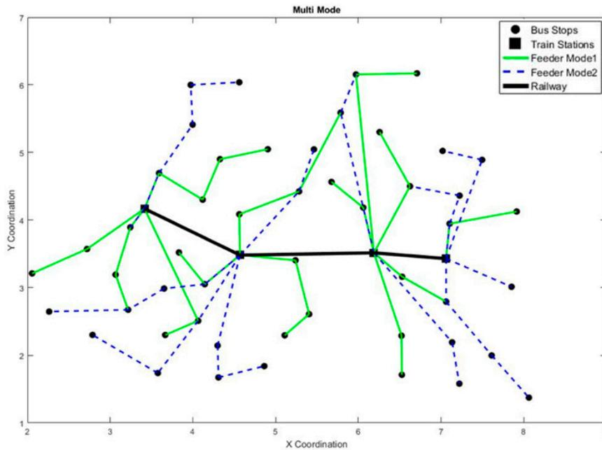
Figure 8. An example of for multimodal feeder network design problems(MFNDP) after demand proportion ratio.
