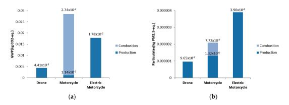
**Figure 6.** GWP and particulates of 1 km delivery by drone, motorcycle, and electric motorcycle. (a) GWP of 1 km delivery; (b) PM<sub>2.5</sub> of 1 km delivery.
