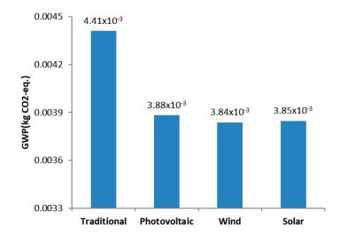
Figure 8. GWP of 1 km drone delivery under renewable energy scenario.
