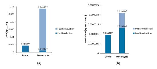
**Figure 3.** Global warming potential (GWP) and particulates matter (PM<sub>2.5</sub>) produced per 1 km delivery by drone and motorcycle. Energy options for drone and motorcycle are electricity and gasoline, respectively. (**a**) GWP; (**b**) PM<sub>2.5</sub>.
