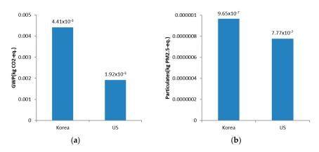
**Figure 7.** GWP and particulates of 1 km delivery distance by drone in South Korea and in the U.S. (**a**) GWP; (**b**) PM<sub>2.5</sub>.
