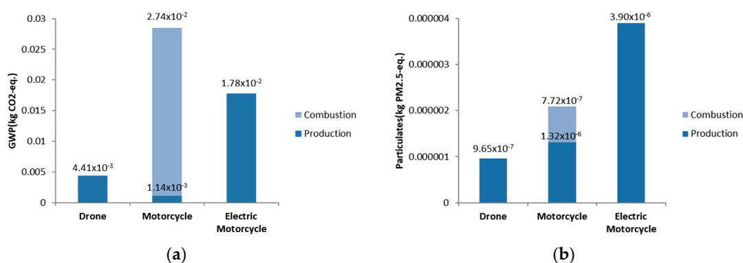
**Figure 6.** GWP and particulates of 1 km delivery by drone, motorcycle, and electric motorcycle. (a) GWP of 1 km delivery; (b) PM<sub>2.5</sub> of 1 km delivery.
