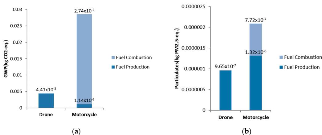
**Figure 3.** Global warming potential (GWP) and particulates matter (PM<sub>2.5</sub>) produced per 1 km delivery by drone and motorcycle. Energy options for drone and motorcycle are electricity and gasoline, respectively. (a) GWP; (b) PM<sub>2.5</sub>.
