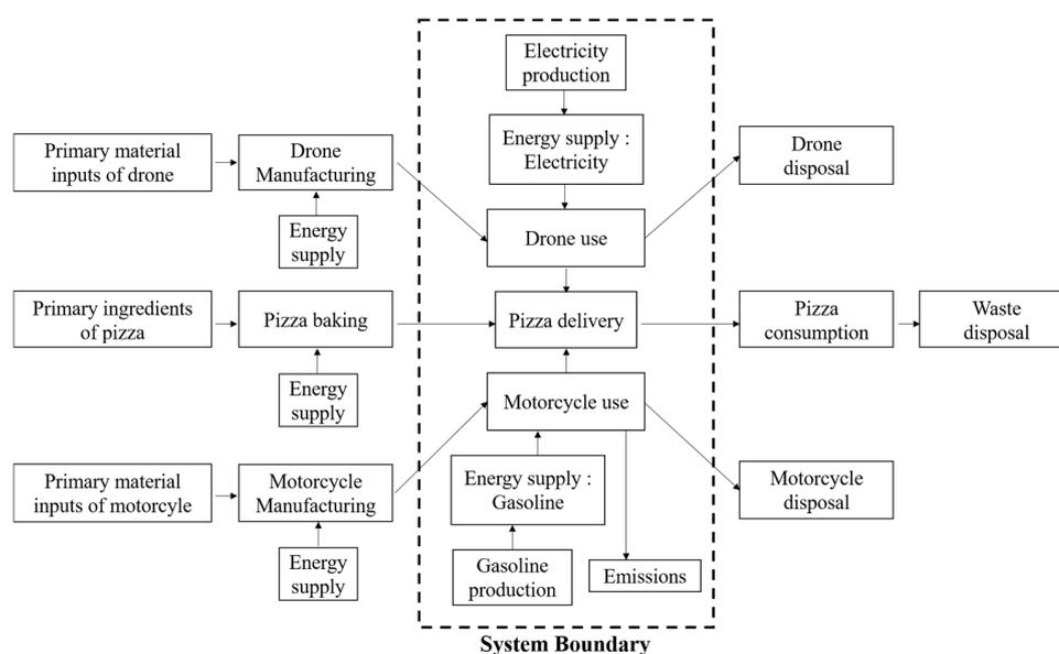
Figure 2. System boundary of a food (pizza) delivery system for drone and motorcycle.
