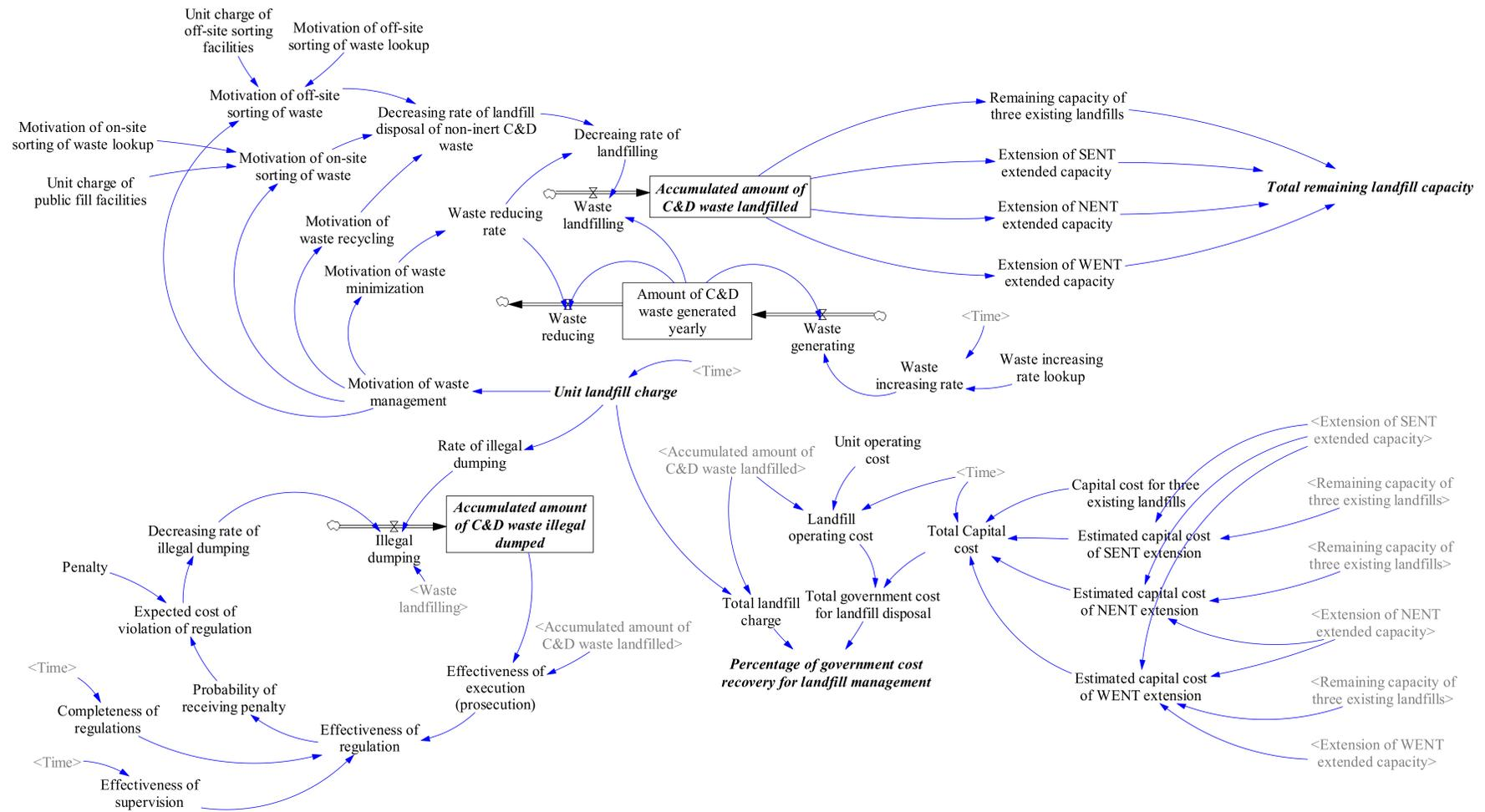
Figure 5. Final stock-and-flow diagram.
