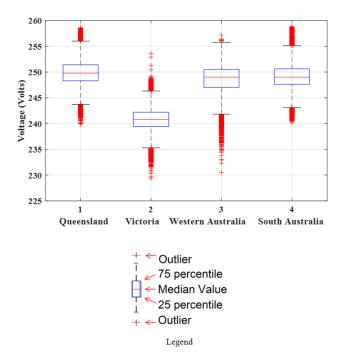
Figure 2. Voltage Box and Whisker Plot (minute wise).
