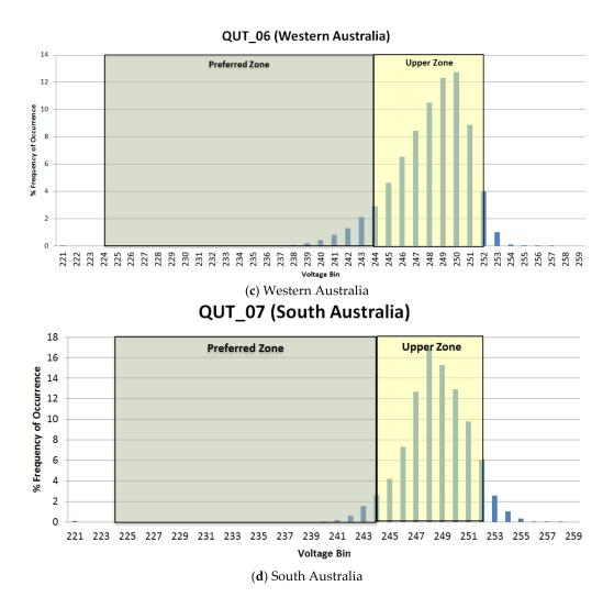
Figure 3. (a–d) Voltage Variation in each location according to AS61000.3.100.
