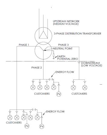
**Figure 11.** Representation of energy flows and unbalanced phase distribution on a low-voltage (LV) network.
