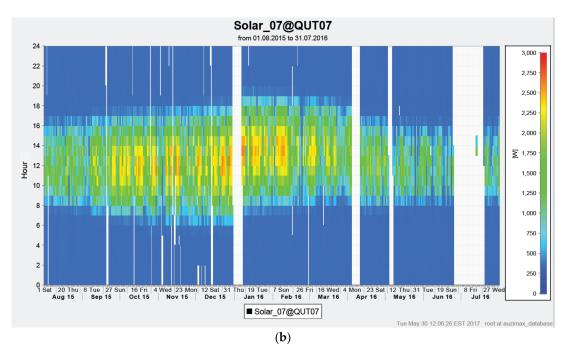
**Figure 7.** (a) Carpet graph of solar generation for Queensland case study; (b) Carpet graph of solar generation for South Australian case study.
