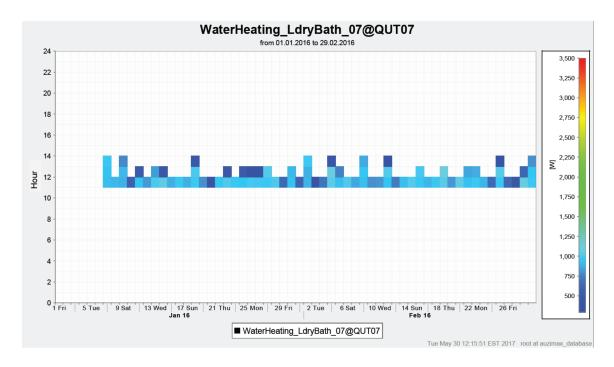
Figure 10. Carpet graph of heat pump hot water service in South Australian house.
