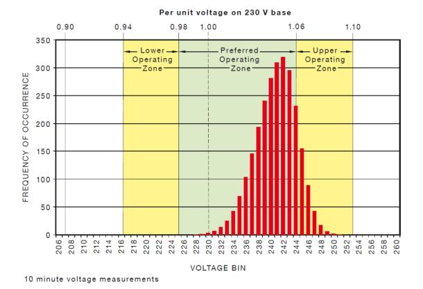
Figure 1. Example of voltage distribution based on AS 61000.3.100 (230 V) [45].
