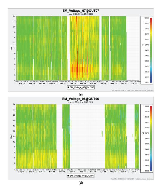
**Figure 4.** Voltage variation carpet graphs for case study house in (a) Queensland; (b) South Australia; (c) Victoria; (d) Western Australia.
