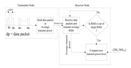
Figure 2. Block diagram of the 5G-based Transmission Power Control (TPC) in Fog and IoT system.
