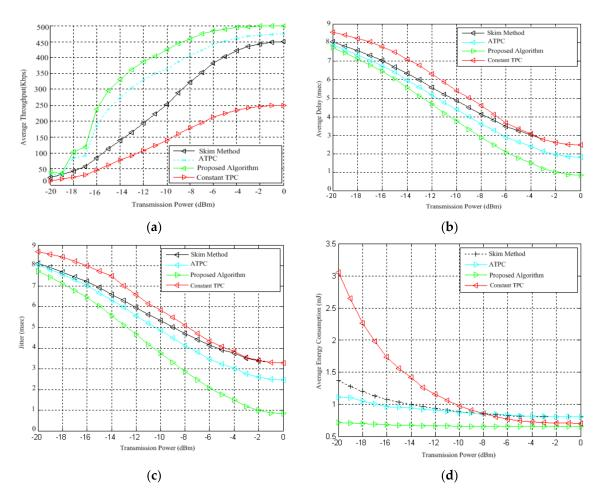
**Figure 6.** Transmission power vs. network metrics (**a**) Average throughput, (**b**) average delay, (**c**) jitter, (**d**) average energy consumption.
