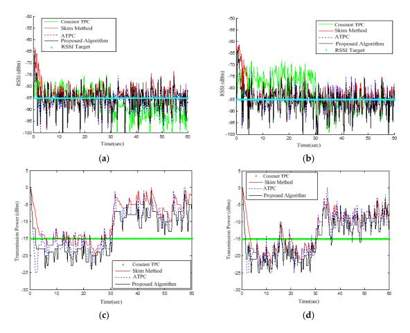
**Figure 5.** Transmission power level and Received Signal Strength Indicator (RSSI) in Dynamic and Static Channel states (a) and (c) Transmission power level, (b) and (d) RSSI of each data packet.
