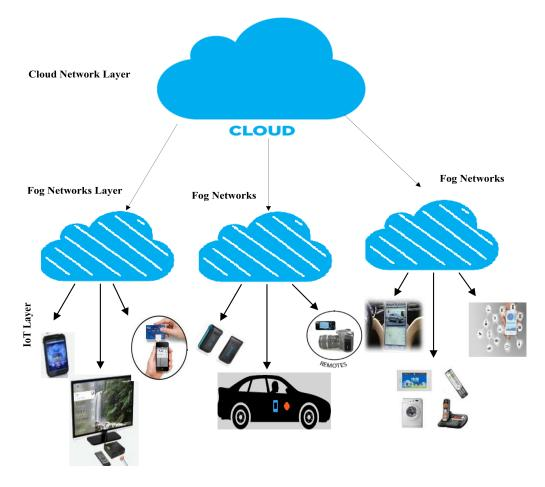
Figure 1. Proposed 5G-enabled Fog Computing and Internet of Things (IoT) based Architecture.
