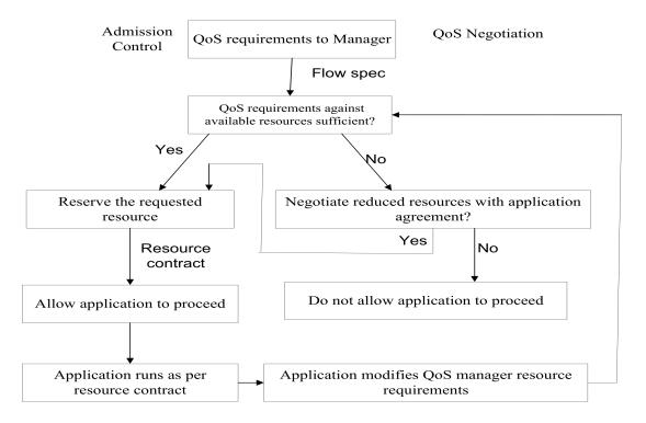
Figure 3. Flowchart of the Quality of Service (QoS) requirement in Fog and IoT systems.
