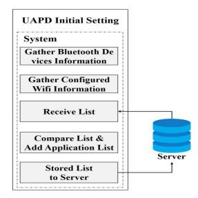
Figure 7. UAPD Initial Setting process.
