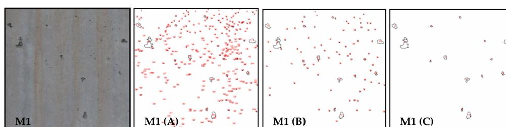
**Figure 7.** From left to right: Image of M-1 and results with filters 1 × 1 (A), 2 × 2 (B) and 5 × 5 (C).
