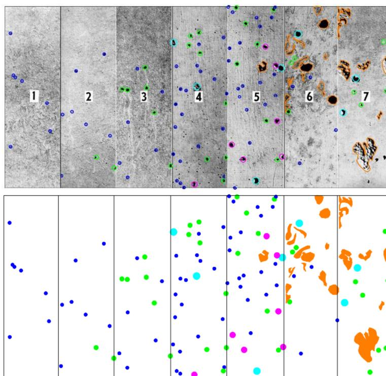
Figure 9. Application of the QSI method and ImageJ on the templates of the CIB W29 code.
