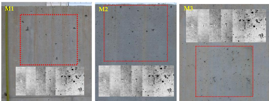
Figure 15. Inspection done with the CIB method on M-1, M-2 and M-3 (from left to right).
