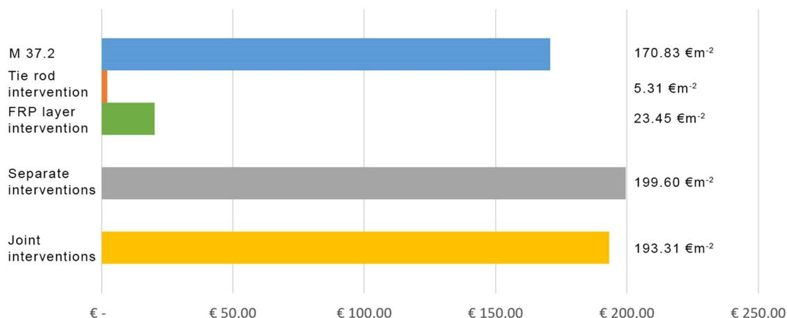
**Figure 16.** Cost of interventions graph. The blue bar represents the cost for the energy retrofit M 37.2; the orange bar is the cost for the seismic retrofit (tie rod); the green bar represents the cost for the seismic retrofit (one FRP layer); the grey bar is the cost for three separated interventions (M 37.2, tie rod, FRP layer); and the yellow bar represents the cost for three joint interventions (M 37.2 + tie rod + FRP layer).
