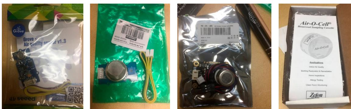
**Figure 21.** From the left: an air quality detection sensor, a formaldehyde detector, a CO<sub>2</sub> detector and bio-aerosol cassettes.
