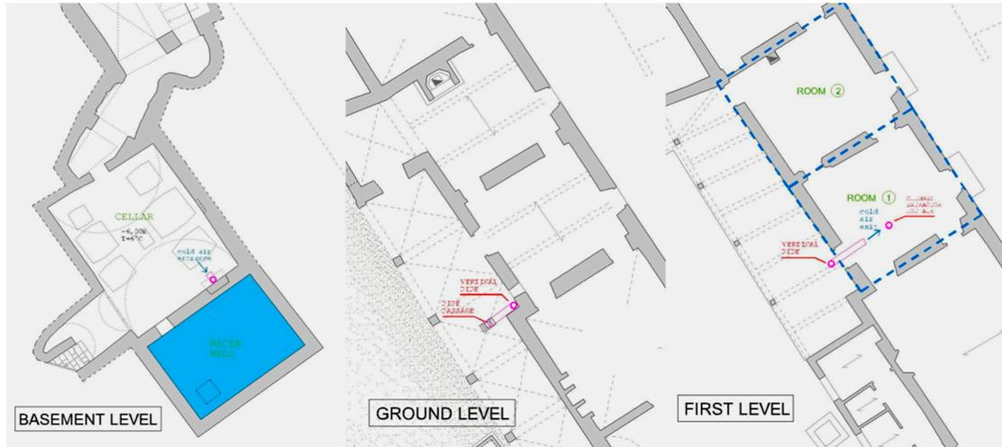
**Figure 8.** Model of the ventilation path through the various levels (underground, ground floor and first floor).
