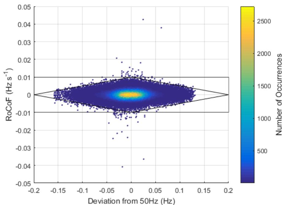
Figure 5. RoCoF versus frequency deviation from 50 Hz.
