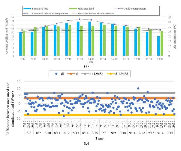
**Figure 20.** Comparison of simulated and actual building cooling loads of the office building. (**a**) Time-varying loads and (**b**) consistency validation.
