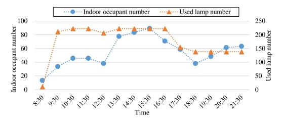
Figure 13. Time-varying used lamp number corresponding to indoor worker number in the office building.
