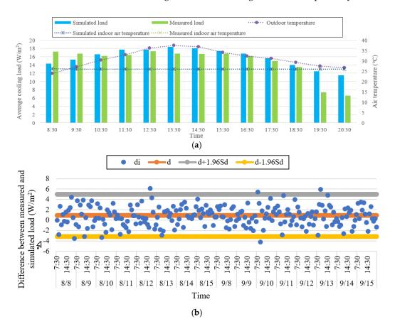
**Figure 19.** Comparison of simulated and actual building cooling loads of the teaching building. (a) Time-varying loads and (b) consistency validation.
