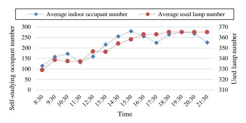
Figure 12. Time-varying used lamp number corresponding to self-studying occupant number.
