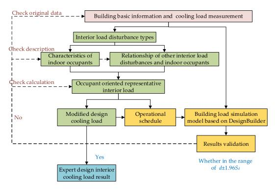
Figure 1. Occupant-oriented, representative interior load establishment and application procedure.
