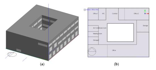
**Figure 17.** Building cooling load simulation model based on DesignBuilder of the office building. (a) External view and (b) interior division of standard floor.
