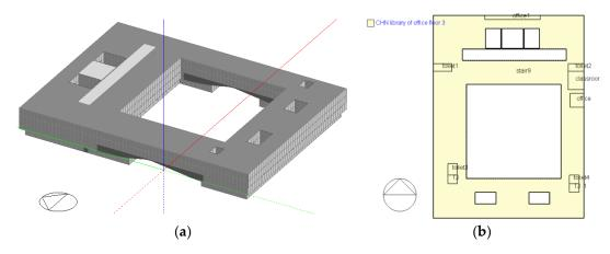
**Figure 18.** Building cooling load simulation model based on DesignBuilder of the library. (**a**) External view and (**b**) interior division of standard floor.
