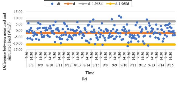
**Figure 21.** Comparison of simulated and actual building cooling loads of the library. (**a**) Time-varying loads and (**b**) consistency validation.
