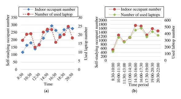
**Figure 14.** Time-varying used laptop number corresponding to self-studying occupant number. (a) Teaching building; (b) Library.
