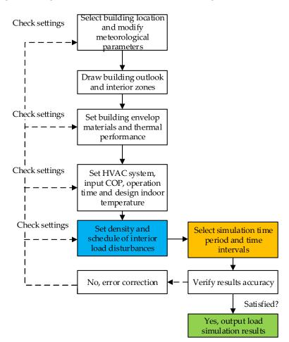
Figure 2. Flow chat of building load simulation based on DesignBuilder tool.
