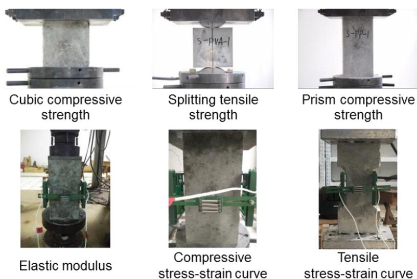
Figure 4. Mechanical property test setups.
