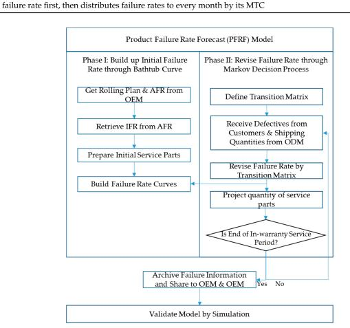
Figure 4. The Product Failure Rate Forecasting (PFRF) Model.
