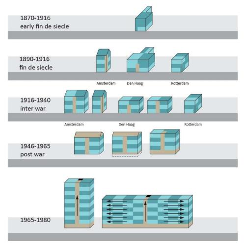
Figure 4. Typology of the Dutch tenement apartment building. Graphic by Leo Oorschot.
