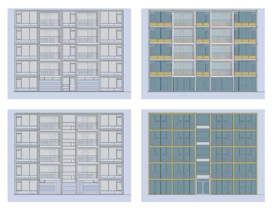
**Figure 7.** VAM walk-up apartment building (1960) with characteristic façade of dry assemblage of prefabricated construction components as concrete façade elements and window frames. **Top left:** original street façade; **below left:** original garden façade. **Top right:** adaptions on in the new design; **below right:** glass covered balcony and extension.
