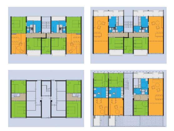
**Figure 6.** VAM walk-up apartment building (1960) with type E3 floorplan. **Top left**: original plan 2e, 3e, and 4e floors. **Bottom left**: original ground floor. **Top right**: new plan 2e, 3e, and 4e floors. **Bottom right**: new plan ground floor. Drawing Leo Oorschot.
