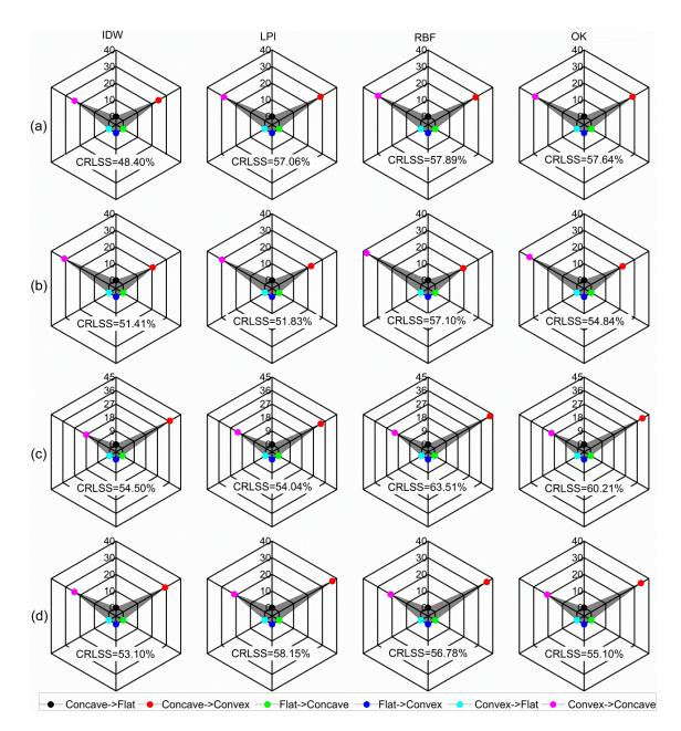
**Figure 13.** CRLSS of the surface models of different geomorphic subunits: (**a**) lagoon slope, (**b**) lagoon bottom, (**c**) deep patch reef, and (**d**) shallow patch reef. The six colors in the figure represent the changes among the three different local slope shapes, and the size of the shaded area represents the ratio of the changes of different local slope shapes.
