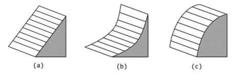
Figure 3. Schematic diagram of local slope shapes: (a) flat slope, (b) concave slope, and (c) convex slope.
