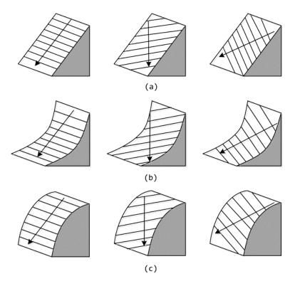
**Figure 4.** Schematic diagram of local slopes with different aspects: (**a**) flat slope with different aspects, (**b**) concave slope with different aspects, and (**c**) convex slope with different aspects.
