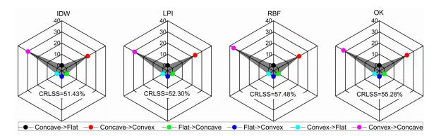
**Figure 10.** Change rate of the local slope shape (CRLSS) of the surface models with 1-m resolution were reconstructed by (**a**) IDW, (**b**) LPI, (**c**) RBF, and (**d**) OK. The six colors in the figure represent the changes among three different local slope shapes, and the size of the shaded area represents the ratio of the changes of different local slope shapes.
