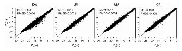
**Figure 9.** Root mean square error (RMSE) of the surface models with 1-m resolution were reconstructed by (a) IDW, (b) LPI, (c) RBF, and (d) OK:  $Z_e$  represents the estimated value and  $Z_o$  represents the observed value.
