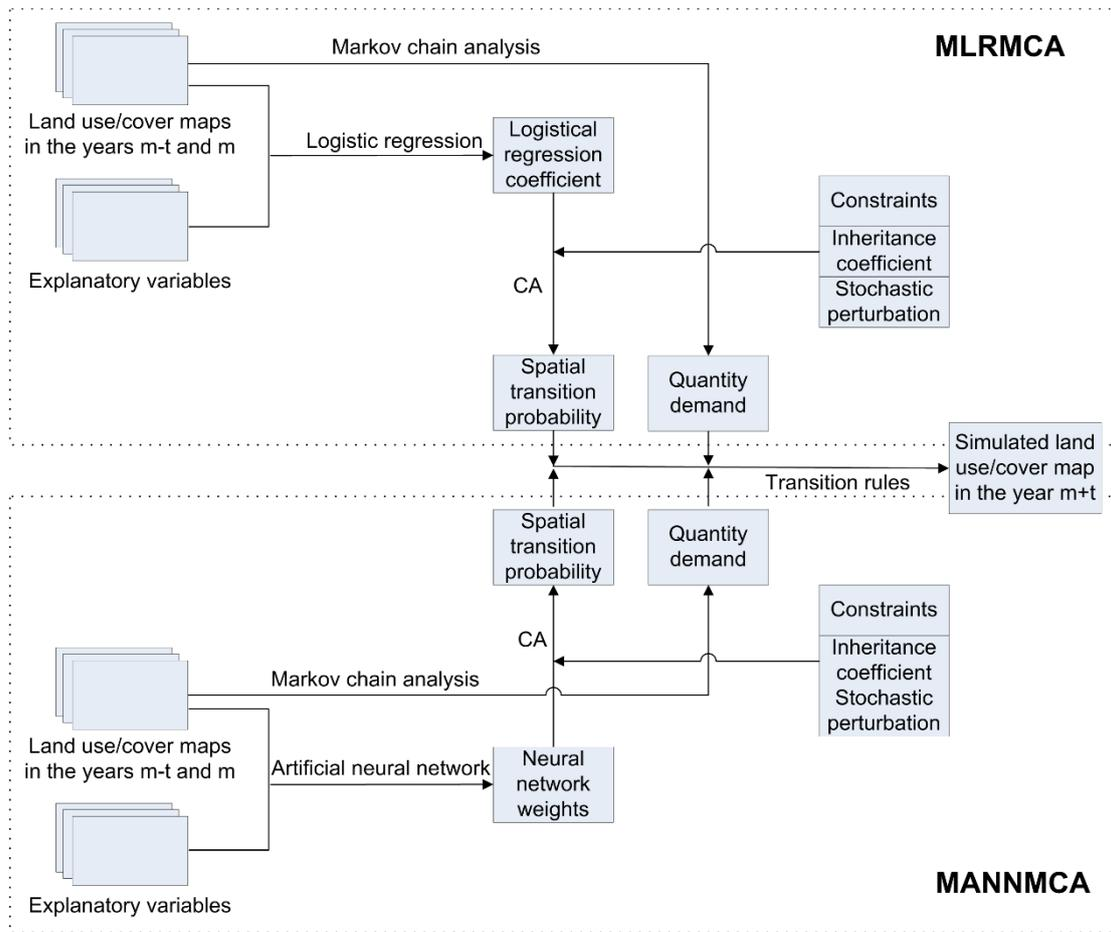
**Figure 1.** Structure of the multiple logistic regression cellular automata (MLRMCA) model and the multiple artificial neural network cellular automata (MANNMCA) model.
