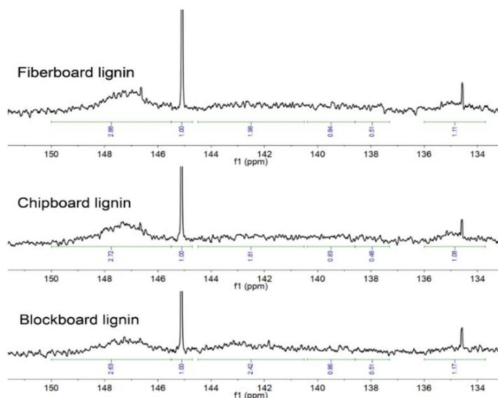
**Figure 4.** Quantitative <sup>31</sup>P NMR spectra of the three PHP technical lignins.
