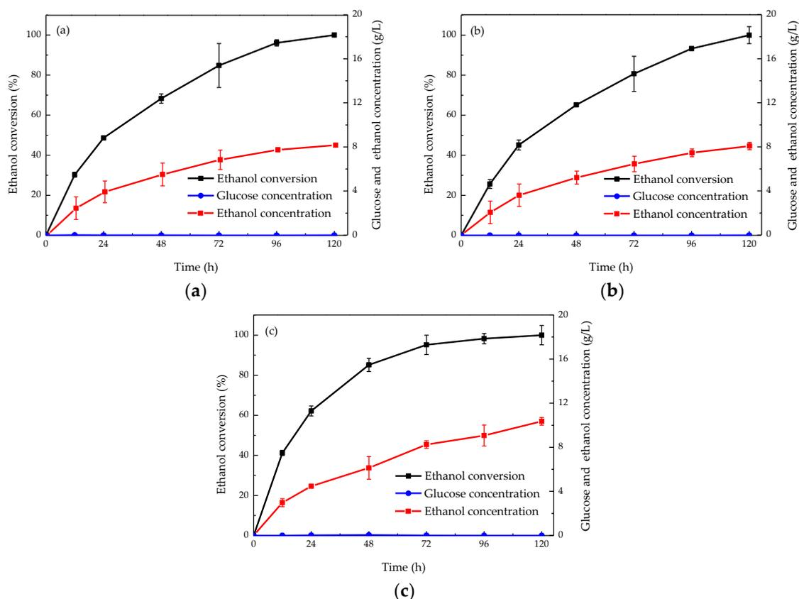
**Figure 3.** Glucose and ethanol concentrations and ethanol conversion in simultaneous saccharification and fermentation (SSF): (a) fiberboard, (b) chipboard, and (c) blockboard.
