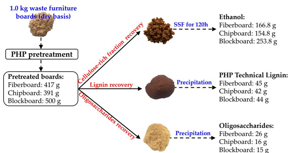
Figure 5. Overall mass balance of PHP pretreatment on the three furniture boards.
