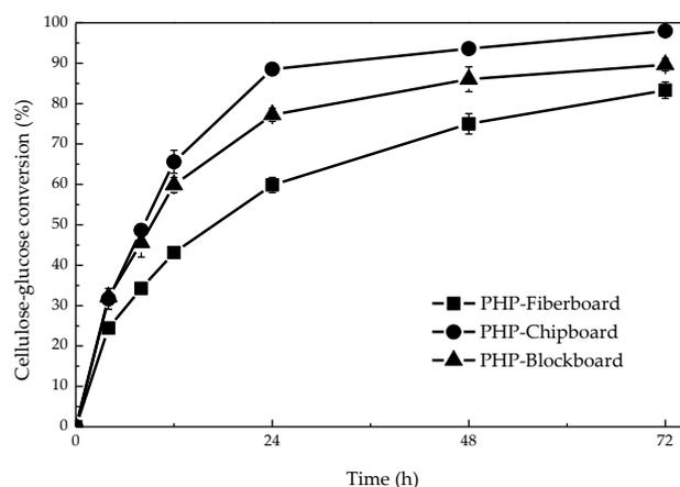
**Figure 1.** Enzymatic hydrolysis of the three furniture boards after pretreatment.
