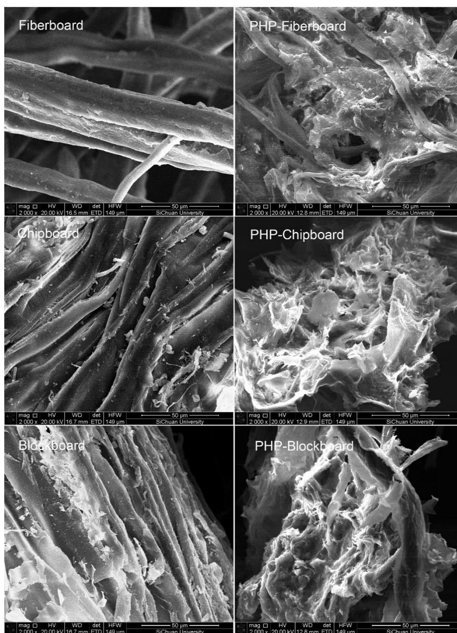
**Figure 2.** SEM micrographs of the furniture boards and pretreated substrates at 2000× magnification.
