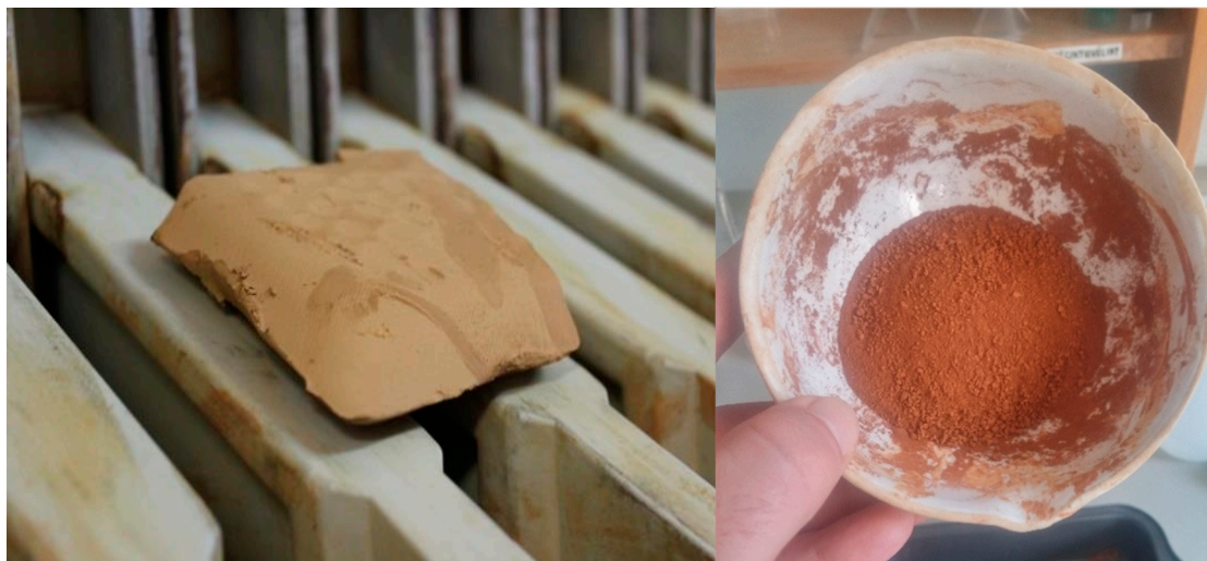
Figure 1. The water treatment iron sludge and the iron sludge powder.
