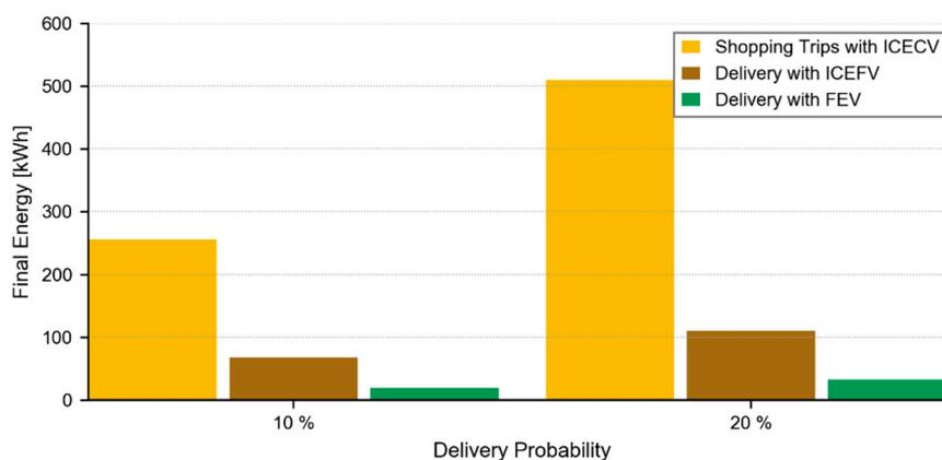
**Figure 6.** Potential to save energy by the delivery of groceries in Haidhausen Süd for different drive types of delivery vehicles (Customer Vehicles: ICECV; share of private vehicles use for shopping trips, 46.5 %).
