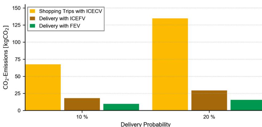
**Figure 7.** Potential to save CO<sub>2</sub> emissions by the delivery of groceries in Haidhausen Süd for different investigated drive types of delivery vehicles (Customer Vehicles: ICECV; share of private vehicles use for shopping trips, 46.5%).
