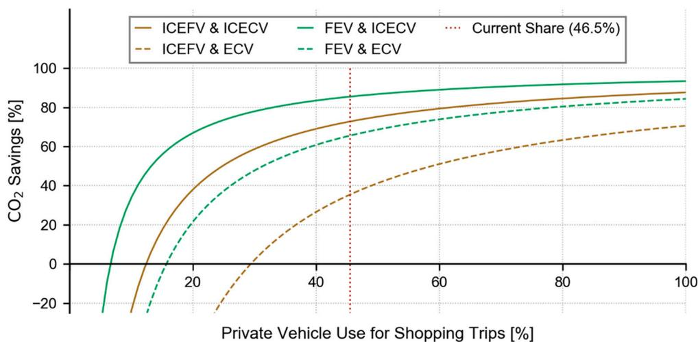
**Figure 10.** CO<sub>2</sub> savings caused by a delivery of groceries as a function of the percentage of vehicle use for individual shopping trips (Delivery Probability 10%).
