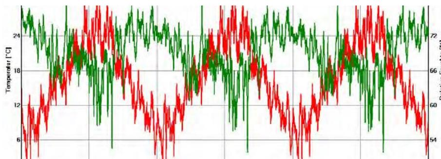
**Figure 10.** Temperature and moisture curve on the internal surface of an energetic renovated Black Sea House in Varna with a back flow of  $1 \text{ m}^3/\text{m}^2\text{h}$  [7].
