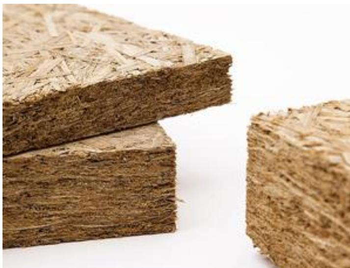
**Figure 2.** TYPHABOARD, picture: Fraunhofer IBP.
