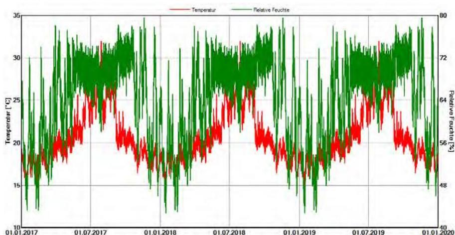
**Figure 9.** Temperature and moisture curve of the interior plaster of an unrenovated Black Sea House in Varna [7].
