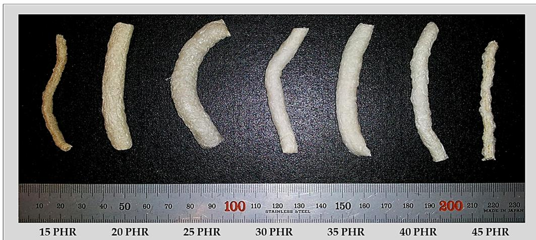
Figure 9. Appearance of foamed cushioning material by water content in a mixing ratio of PP50/WB50.
