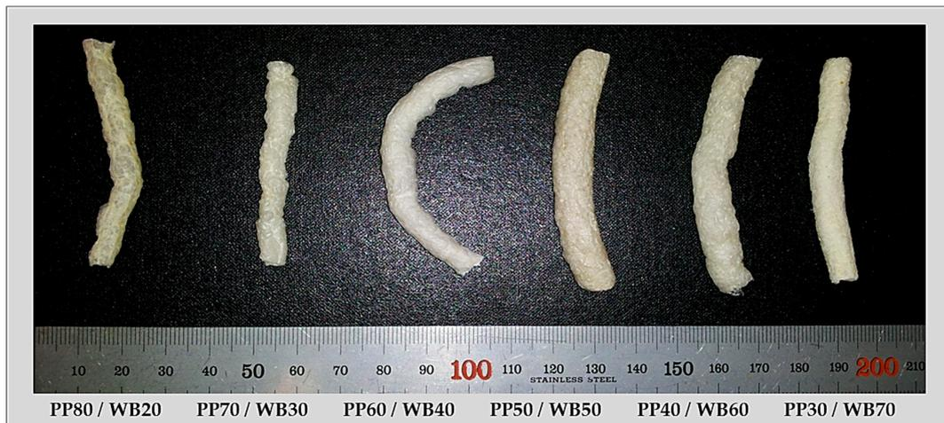
**Figure 8.** Appearance of foamed cushioning material according to the PP and WB mixing ratio, when the water content was 20 PHR.
