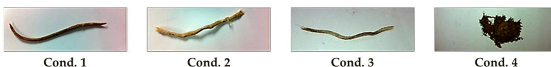
**Figure 5.** Comparisons of the discharged state, according to the extruder temperature conditions under experimental conditions of polypropylene (PP)70/wheat bran (WB)30.
