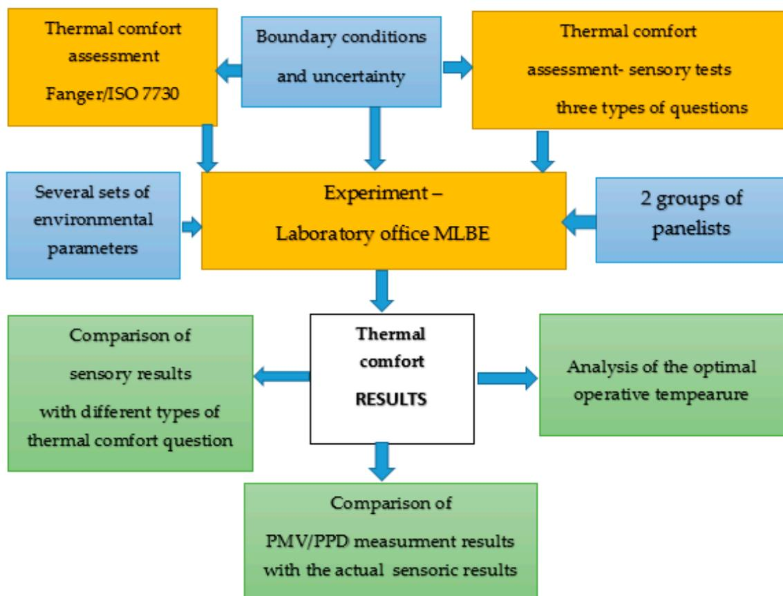
Figure 1. Scheme of the thermal comfort assessment experiment.
