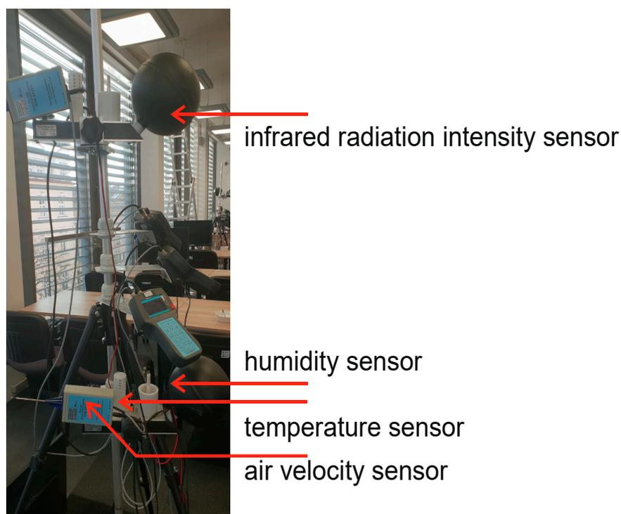
**Figure 5.** The sensors connected to the testing device EHA-MM101 dedicated to thermal comfort measurements (M1).
