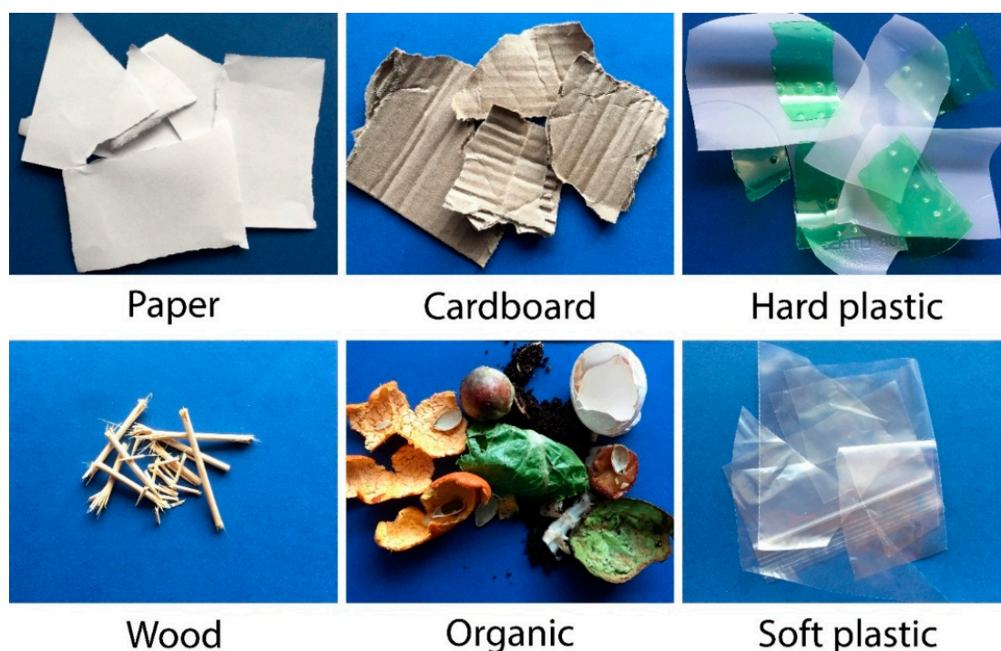
Figure 1. Picture of the collected fractions. These wastes were dried, ground and blended to prepare the RDF samples.
