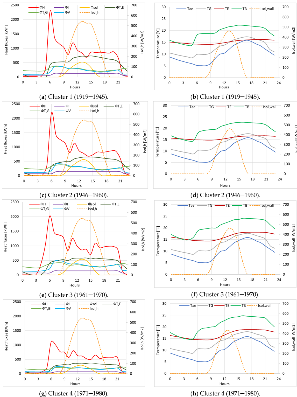
Figure 7. Heat flux components and building temperatures with a variable number of air changes per hour (in daytime ach = 0.62 \text{ h}^{-1} , and in nighttime ach = 0.3 \text{ h}^{-1} ) for a typical day: February 22nd 2014, with a T_{ae} = 6.24 \text{ }^{\circ}\text{C} (clusters for the four construction periods).
