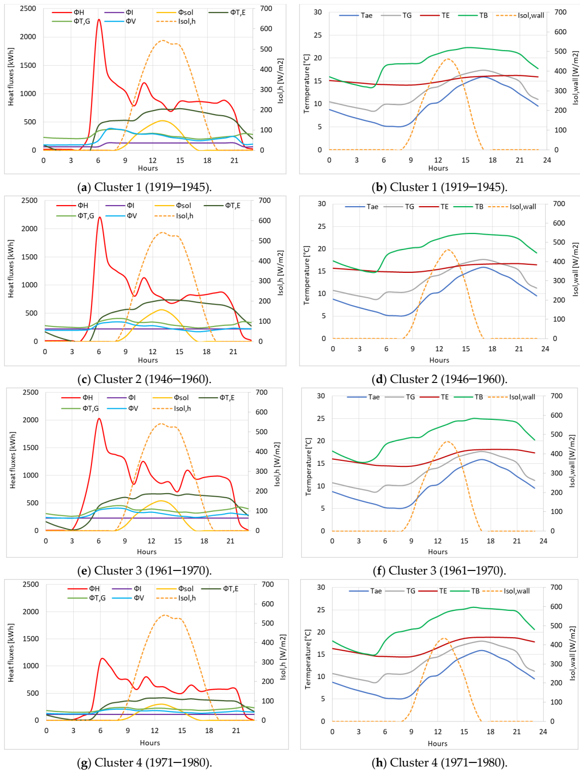
Figure 6. Heat flux components and building temperatures (with constant ach = 0.5 \text{ h}^{-1} ) for a typical day: February 22nd 2014, with a T_{ae} = 6.24 \text{ }^{\circ}\text{C} (clusters for the four construction periods).
