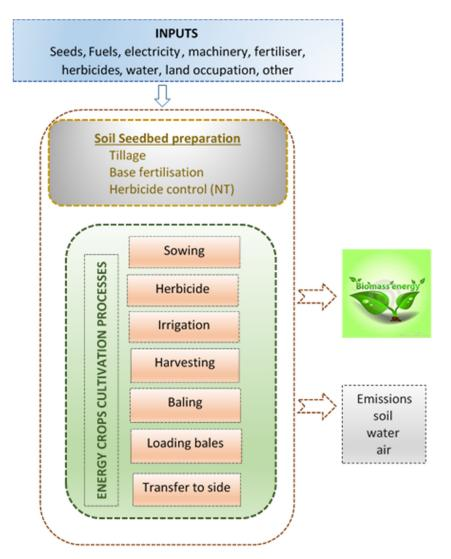
Figure 2. The processes included to the system boundaries for the biomass production.
