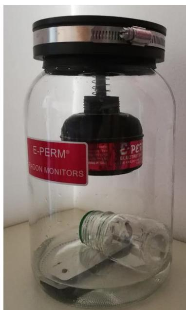
**Figure 4.** Picture of the jar containing the 140 mL bottle and the opened-suspended E-Perm chamber.
