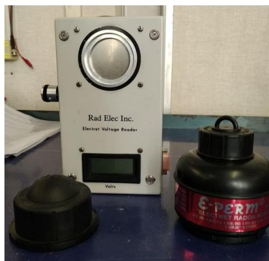
**Figure 2.** Picture of the electrometer (Rad. Elec. Inc. Mod. 6383-01, Frederick, MD, USA) and one Long (on the **left**) and one Short (on the **right**) electret passive environmental radon monitor (E-Perm) chamber.
