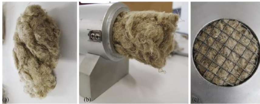
Figure 10. Hemp fibers for impedance tube measurement: (a) loose hemp fibers, (b) hemp fibers within the test rig, and (c) metallic mesh used to restrain the fibers in sample holder [62]. Reproduced with permission from Elsevier Ltd.
