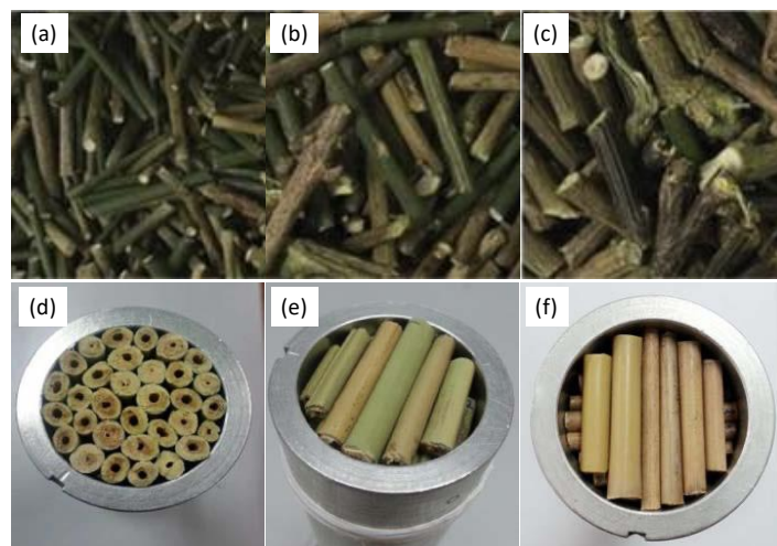
Figure 6. Different diameter broom branches: (a) 1.5 mm, (b) 3 mm, (c) 4 mm, and the arrangement of bamboo in impedance tube: (d) axial arrangement, (e) transverse arrangement, and (f) cross transverse arrangement [54,55]. Reproduced with permission from Elsevier Ltd. and IPPT PAN.
