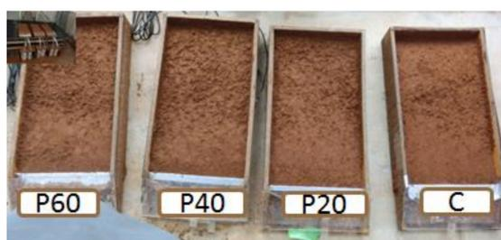
**Figure 8.** Crusts formed on the soil surface after six consecutive storms. Treatments were control (C), PAM of 20 kg ha<sup>-1</sup> (P20), 40 kg ha<sup>-1</sup> (P40), and 60 kg ha<sup>-1</sup> (P60).
