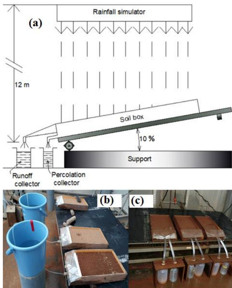
**Figure 1.** Experimental set-up showing (a) rainfall simulator, experimental soil box, and runoff and percolating water collector; (b) different treatments being saturated from below; and (c) runoff and percolating water collection during simulation.
