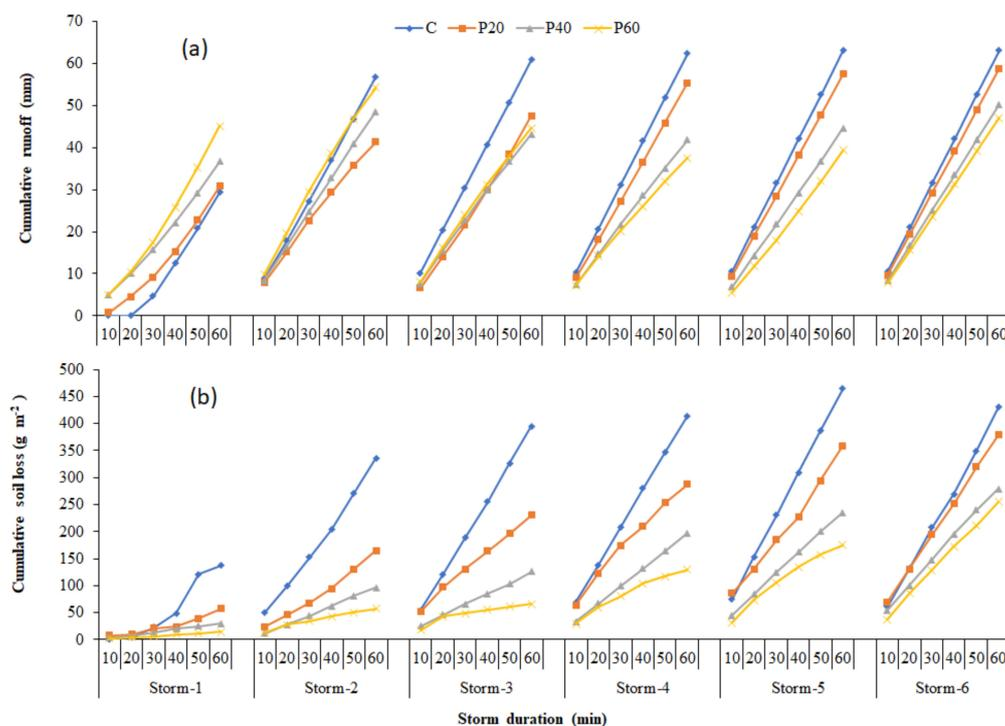
**Figure 4.** Effect of PAM rates on (a) cumulative runoff (mm) and (b) cumulative soil loss ( $\text{g m}^{-2}$ ). Each of the six storms had an average rainfall intensity of  $70 \text{ mm h}^{-1}$  for 1-h duration and 48-h drying period interval. Data were collected at 10-min intervals in the 1-h rainfall duration. The treatments were control (C), PAM of  $20 \text{ kg ha}^{-1}$  (P20),  $40 \text{ kg ha}^{-1}$  (P40), and  $60 \text{ kg ha}^{-1}$  (P60).
