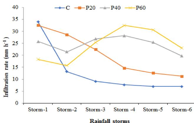
**Figure 3.** Effect of PAM rates on infiltration rate (mm h<sup>-1</sup>). Each of the six storms had an average rainfall intensity of 70 mm h<sup>-1</sup> for 1-h duration and 48-h drying period. The treatments were control (C), PAM of 20 kg ha<sup>-1</sup> (P20), 40 kg ha<sup>-1</sup> (P40), and 60 kg ha<sup>-1</sup> (P60).
