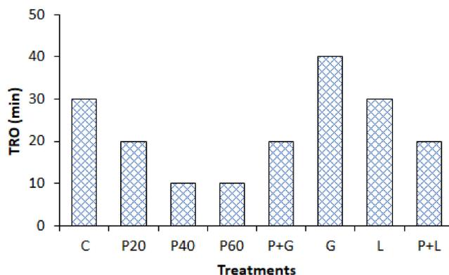
**Figure 2.** Effect of treatments on time to runoff (TRO) for control (C), PAM of 20 kg ha<sup>-1</sup> (P20), 40 kg ha<sup>-1</sup> (P40), 60 kg ha<sup>-1</sup> (P60), PAM of 40 kg ha<sup>-1</sup> + gypsum (4 t ha<sup>-1</sup>) (P+G), gypsum (4 t ha<sup>-1</sup>) (G), lime (2 t ha<sup>-1</sup>) (L), and PAM of 40 kg ha<sup>-1</sup> + Lime (2 t ha<sup>-1</sup>) (P+L).
