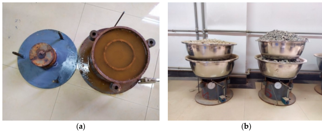
Figure 4. Process of test operation: (a) adding water; (b) applying load.
