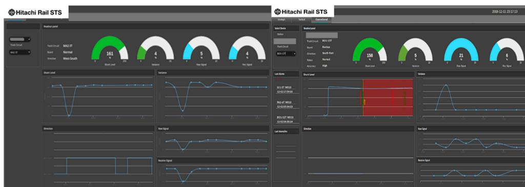
**Figure 9.** HMI dashboard: comparison of track circuits in nominal and out-of-range conditions (detection of anomaly in red).
