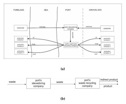
**Figure 7.** Example 4: The supply chain loop for tyres–oil, soot, and scrap metal. (**a**): detailed cargo flow diagram; (**b**): cargo flow model. Source: Compiled by the authors.
