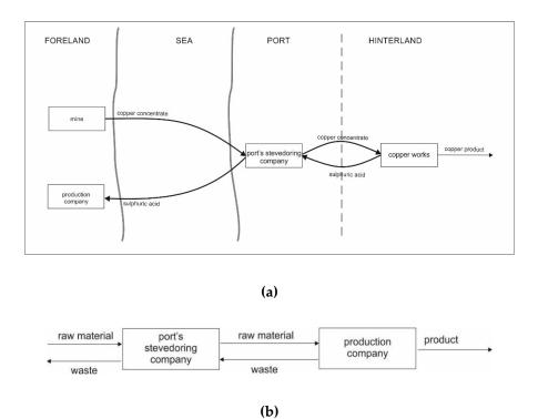
**Figure 5.** Example 2: The supply chain loop for copper concentrate–sulphuric acid. (**a**): detailed cargo flow diagram; (**b**): cargo flow model. Source: Compiled by the authors.
