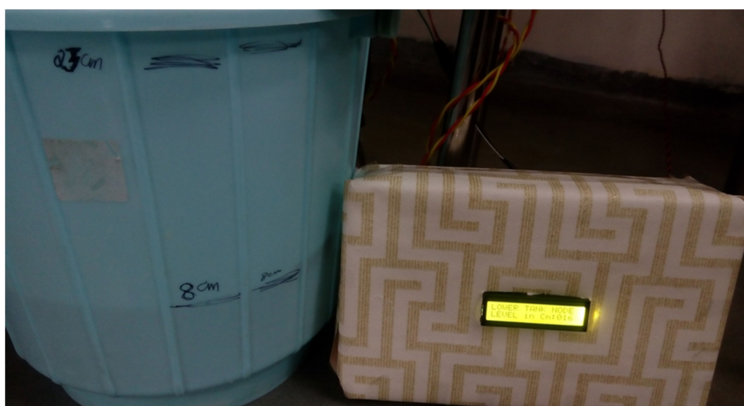
Figure 11. Setup for validation of the Ultrasonic sensor.
