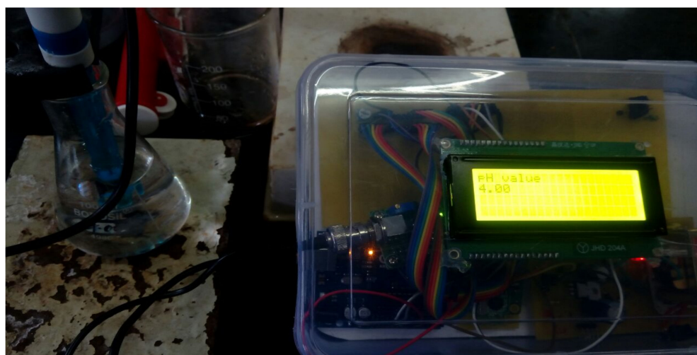
Figure 14. Sensor calibration by 4.00 pH buffer solution.
