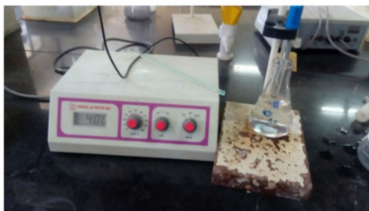
(a) Calibrating the meter to get pH of buffer solution with pH 4.00
