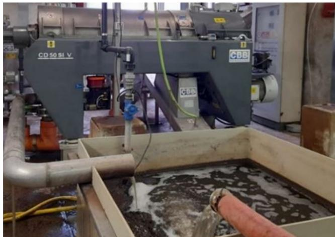
**Figure 3.** Industrial centrifuge to recover SLHC residue.
