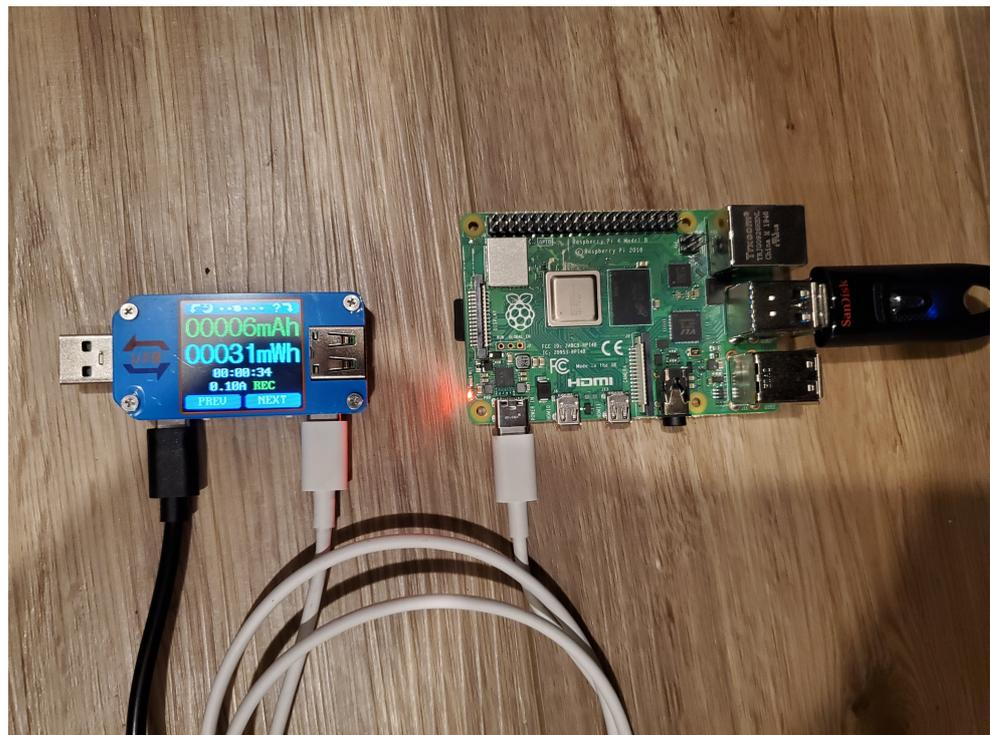
Figure 3. Energy monitoring setup.
