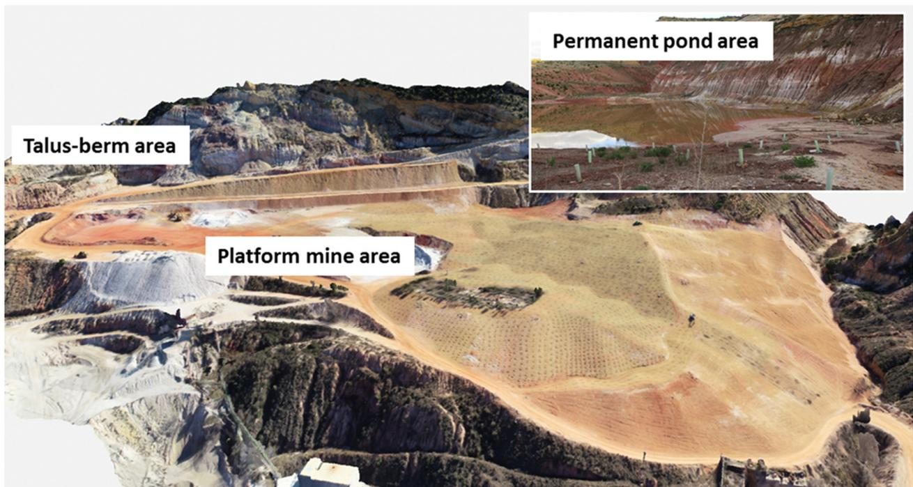
**Figure 2.** General view of the main three areas to be restored (i.e., platform mine area, talus-berm area, permanent pond area), obtained after geomorphological modeling. The Geofluv™ method was performed in the platform mine area, the talus-berm technique was applied due to the presence of steep slopes in the area, and no modeling was carried out in the pond area.
