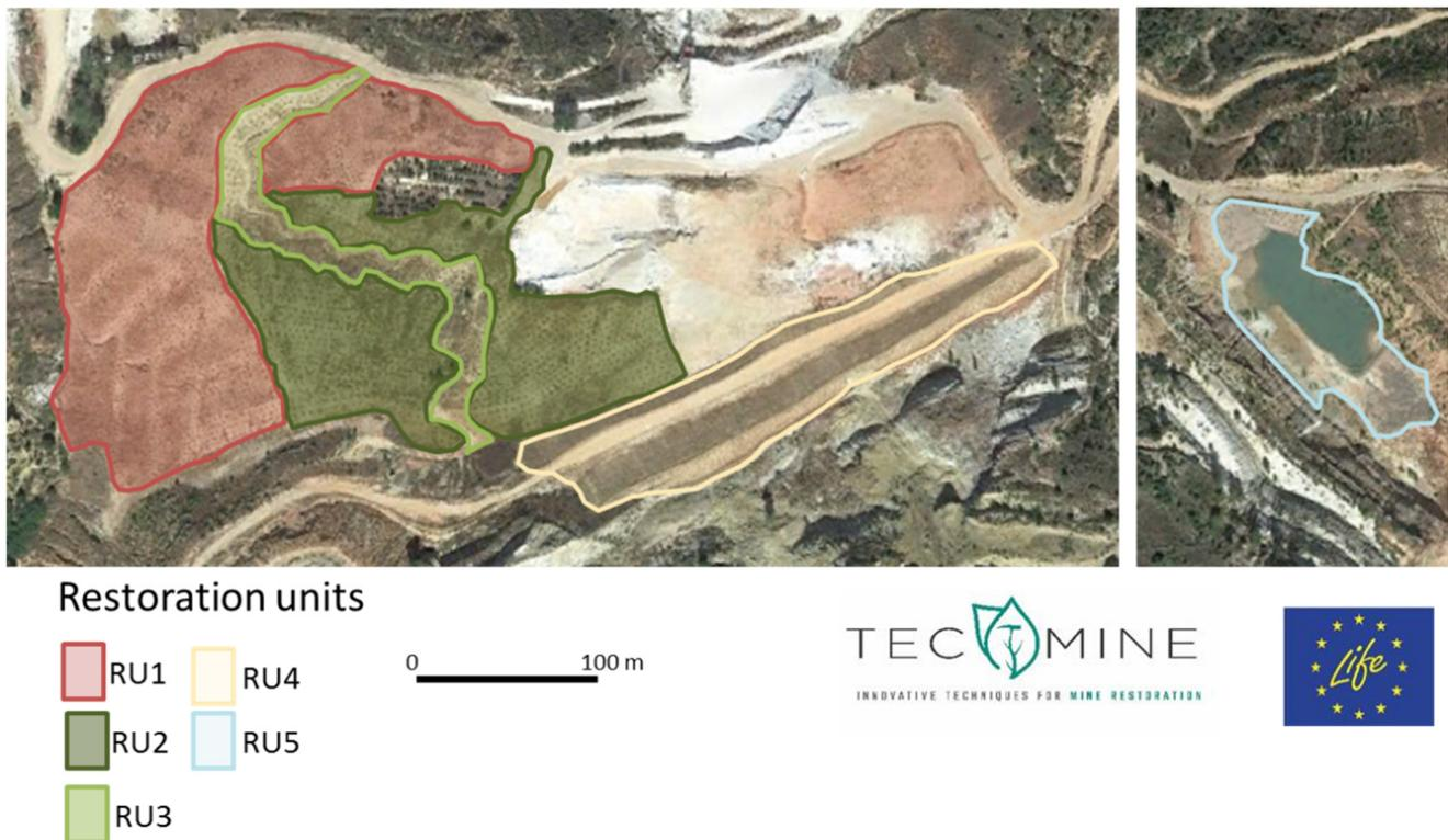
**Figure 4.** Aerial images showing the restored areas and the distribution of restoration units (RUs). Different colored polygons were assigned for each RU. Thus, RU1 is shown in red; RU2 in dark green; RU3 in light green; RU4 in yellow (left); and RU5 in blue (right).
