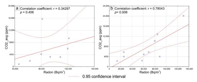
Figure 7. Scatterplots showing relation to radon/ $CO_2$  relation on the West (a) and E side (b) of the fault parallel to the river.
