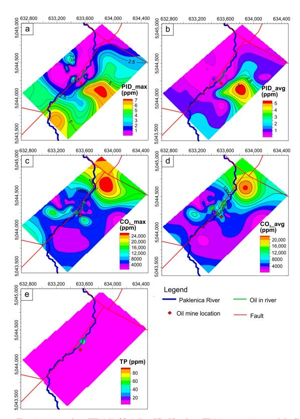
Figure 5. Photo-ionization analyzer (PID) (a,b); CO<sub>2</sub> (c,d); and Total Petroleum (TP) (e) concentrations recorded at Site A.
