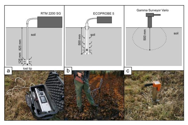
Figure 2. (a) Sarad RTM 2200; (b) ECOPROBE 5; and (c) Gamma Surveyor Vario measuring principles.
