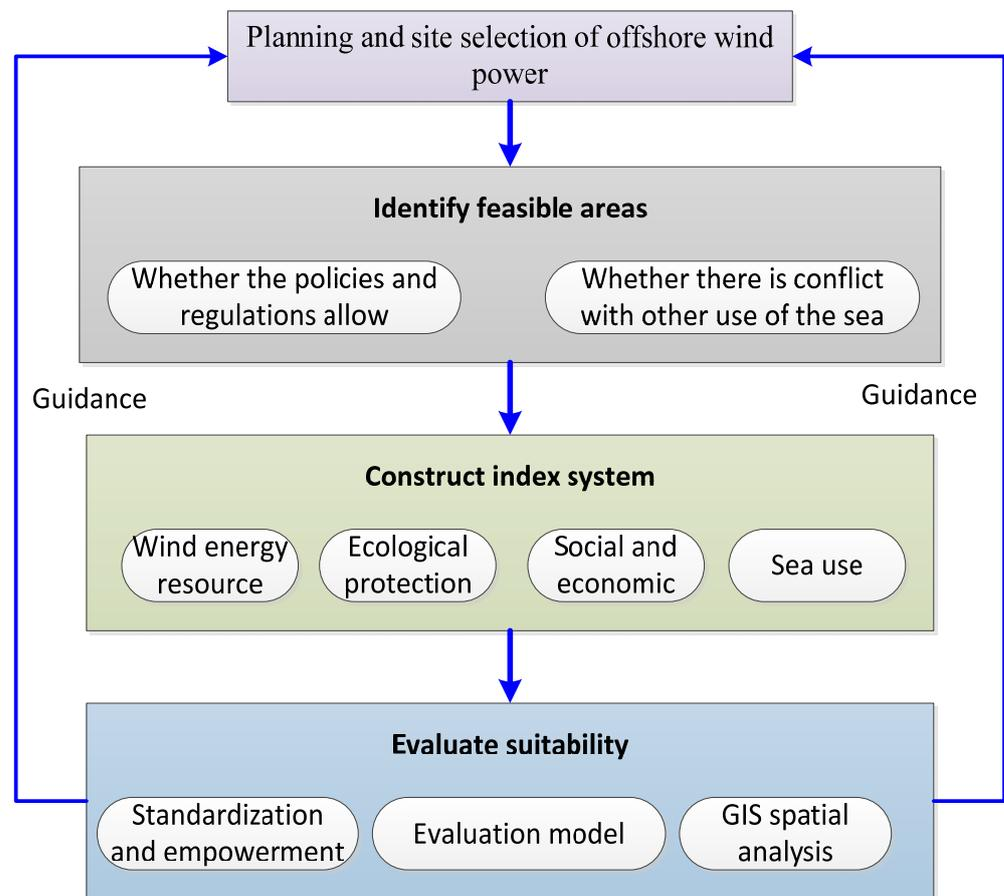
**Figure 2.** Research framework for determining the suitability of a site for offshore wind power.
