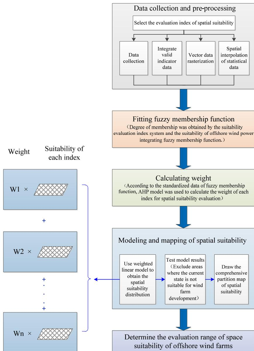
**Figure 3.** Technical roadmap for determining the suitability of a site for offshore wind power.
