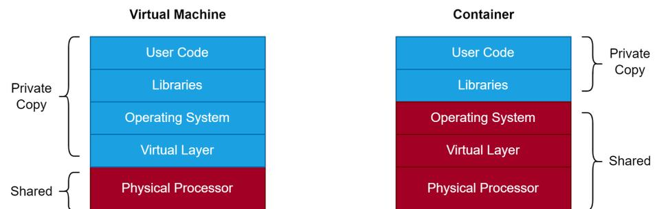
**Figure 1.** Difference in the architecture of virtual machine and container
