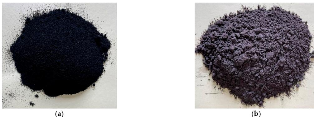
**Figure 1.** Macro appearances of steel slag powder and waste tire rubber. (a) Waste tire rubber powder. (b) Steel slag powder.
