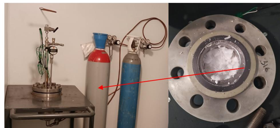
**Figure 1.** Scheme (above) and image (below) of the reactor used for gas hydrates production.
