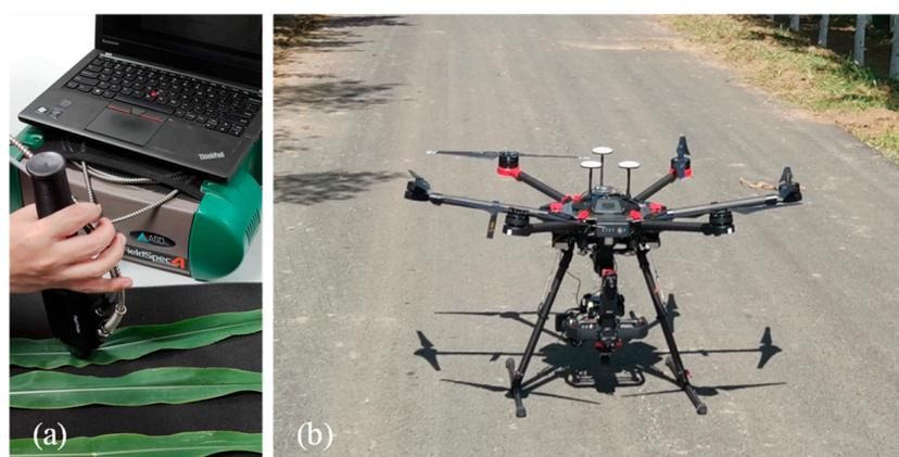
**Figure 1.** Spectral data acquisition using the ground-based (a) and UAV-based (b) sensors.
