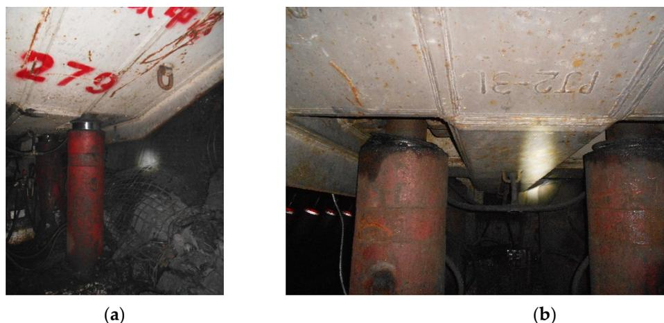
**Figure 1.** Large deformation of roof and hydraulic support crushing accident of a recovery room in Shennan mining area: (a) less than 100 mm stroke of hydraulic support column; and (b) completely crushed hydraulic support.
