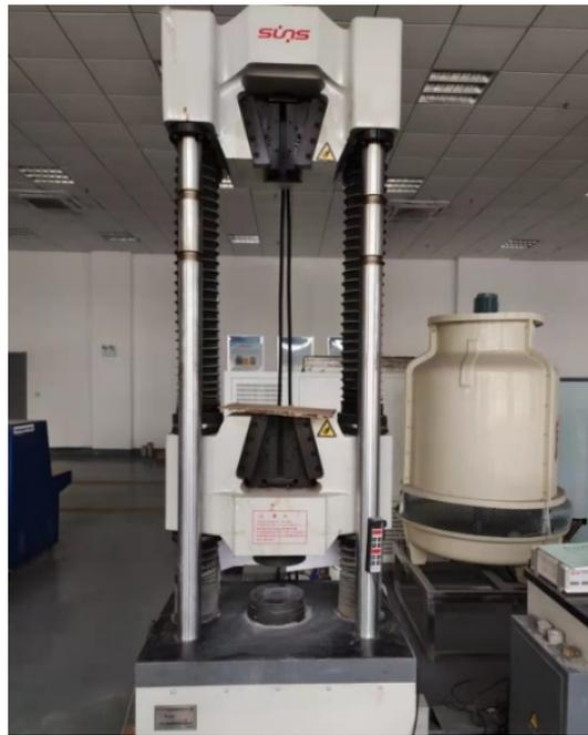
**Figure 4.** WDW-1000 Computer-Controlled Universal Testing Machine.
