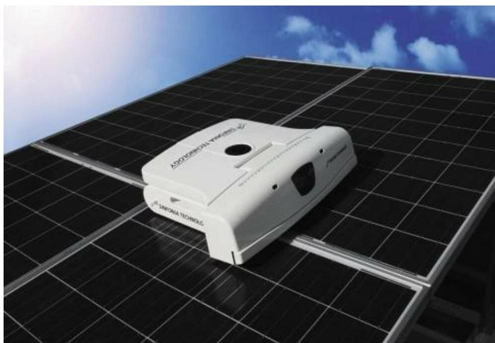
**Figure 2.** Robotic brush cleaning of solar panels [42].
