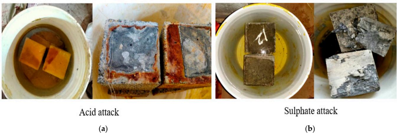
**Figure 13.** (a) Resultant specimen of acid attack test and (b) sulphate attack test. Adapted with permission from Ref. [19]. 2022, Swinburne University of Technology.
