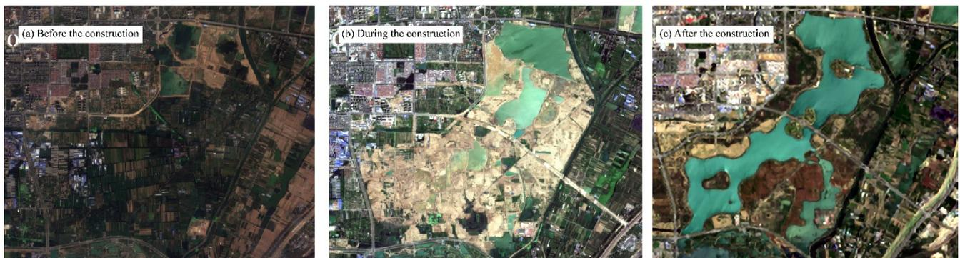
Figure 12. Changes in the treatment process of waterlogging area (the remote sensing images are Sentinel-2 satellite image).
