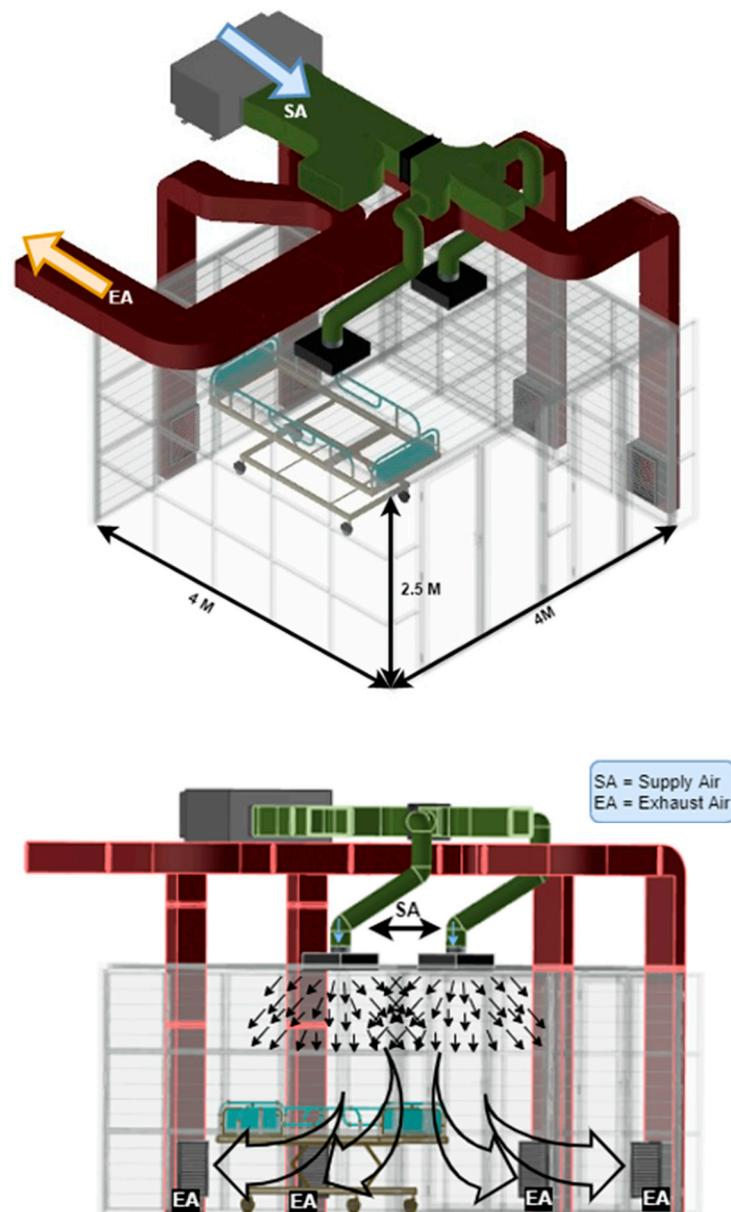
**Figure 2.** Design of heating, ventilation, and air conditioning (HVAC) of the isolation room.
