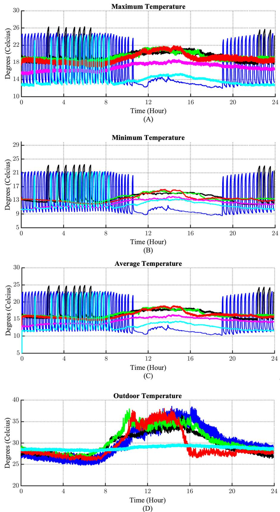
**Figure 11.** The maximum (A), minimum (B), and average (C) temperatures in the patient room for the difference pressure gradient and outdoor (D) temperature.
