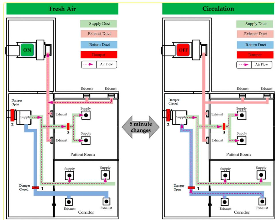
**Figure 7.** The illustration of fresh air/one flow mode and circulation mode within the isolation room.
