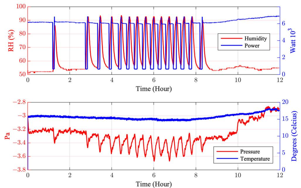
Figure 15. The influence of AC compressor activation to the humidity, pressure, and temperature in the patient room.
