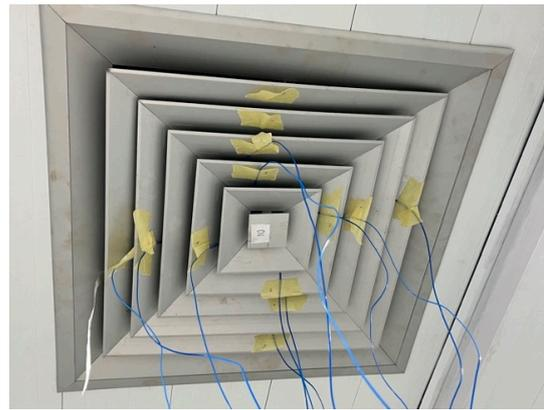
**Figure 4.** Thermocouple arrangement on the supply air grill.
