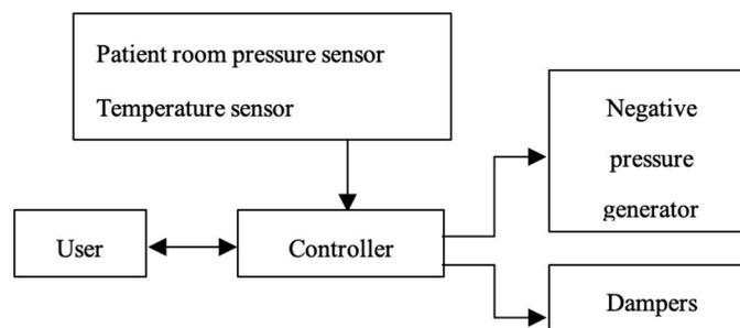
**Figure 5.** Pressure control schematic.
