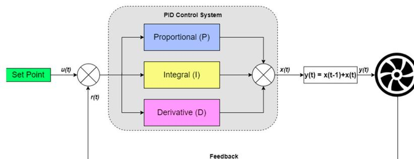
**Figure 8.** PID controller for negative pressure generator.
