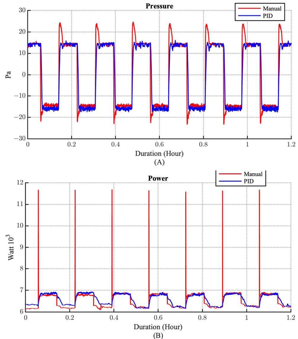
**Figure 9.** Comparison of pressure (A) and power (B) for manual and PID controls.
