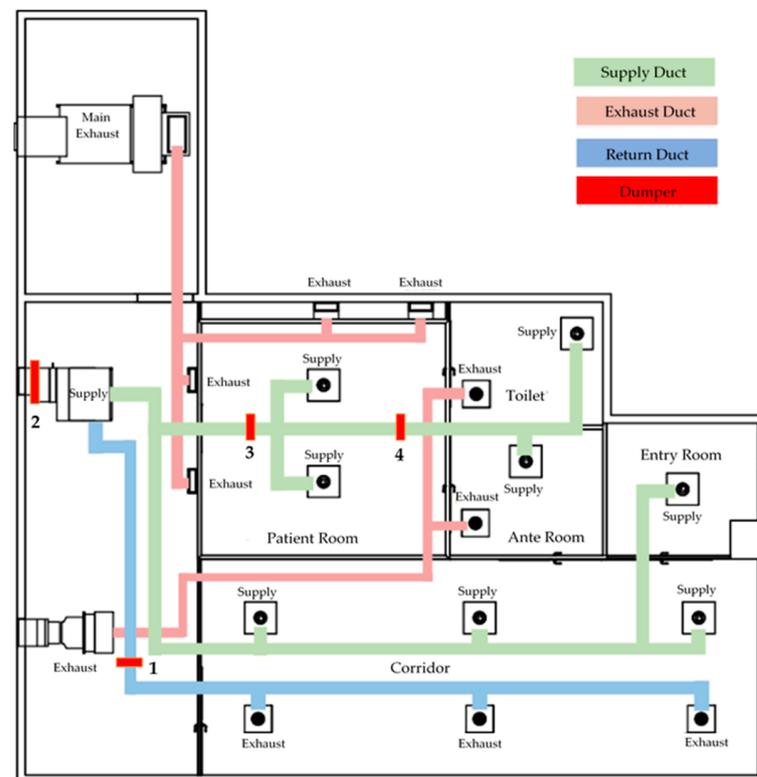
**Figure 1.** Illustration of the isolation room. 1 to 4 are the damper number.
