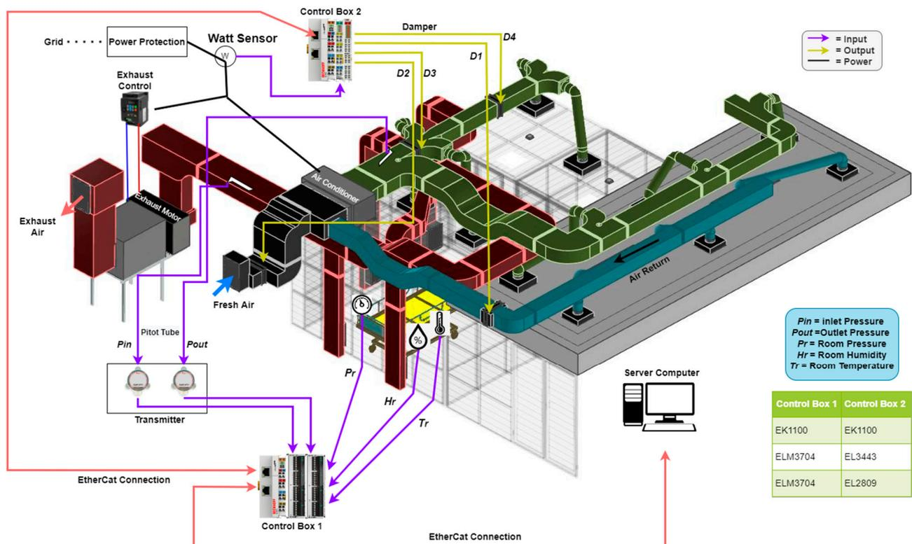
**Figure 3.** Experimental setup for control system testing.
