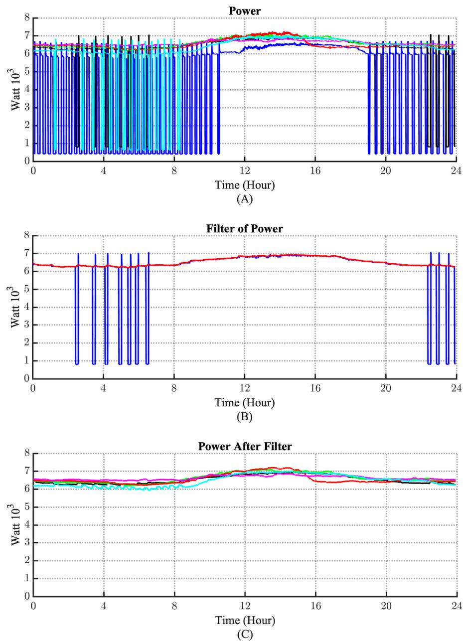
**Figure 12.** The comparison of power measurements (A) for different pressure differentials, during filtering of the power (B), and after filtering (C).
