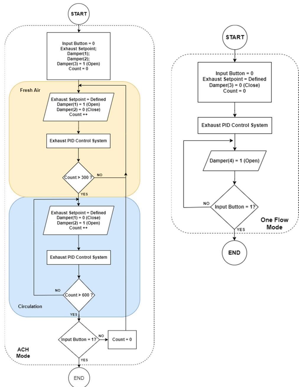
**Figure 6.** Flow chart of the air change per hour (ACH) and one flow mode.
